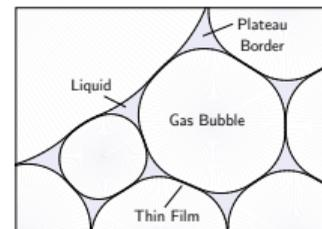
Figure 1: The structure of a two-dimensional wet foam.
