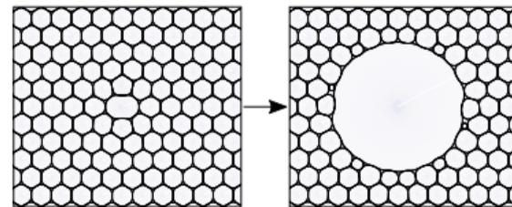
Figure 2: Simulated coarsening of a defective hexagonal foam with liquid fraction  $\phi = 0.056$ .
