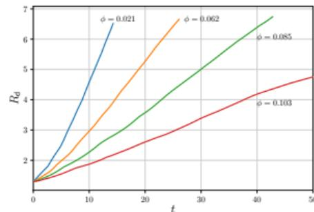
Figure 11: The effective radius of the initially defective bubble against dimensionless time, for several liquid fractions.
