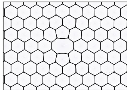
Figure 10: A defective hexagonal foam with liquid fraction  $\phi = 0.021$ . We refer to the large bubble as the **initially defective bubble**.
