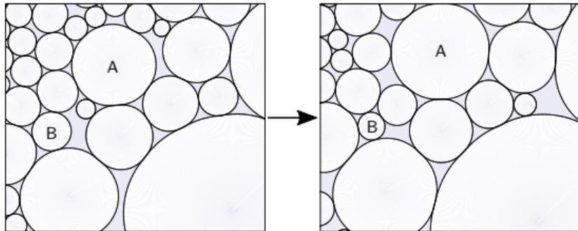
Figure 9: A disordered foam with liquid fraction  $\phi = 0.103$  before and after a period of coarsening.  $A$  is a large bubble that has grown, and  $B$  is a small bubble that has shrunk.
