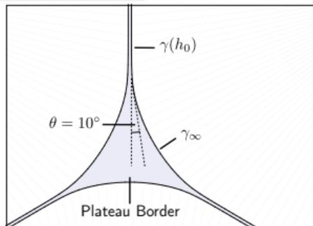
Figure 4: The film-border contact angle  $\theta$  [11]. Our results use  $\theta = 0$ .
