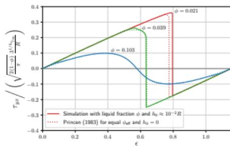
Figure 7: Comparison of simulated stress-strain curves with ref. [12], using 384 vertices.
