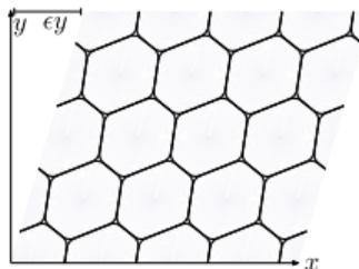
Figure 6: A finite portion of a simply-sheared hexagonal foam, at strain  $\epsilon$  and with liquid fraction  $\phi = 0.02$ . We let  $\epsilon = 0$  correspond to a symmetric state.
