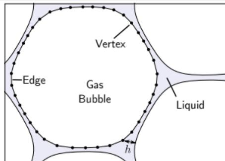
Figure 3: The discretisation in our structural model, including the local film thickness  $h$ .
