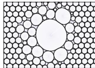
Figure 15: Foam with  $\phi = 0.103$  coarsened to dimensionless time  $t = 50$ .
